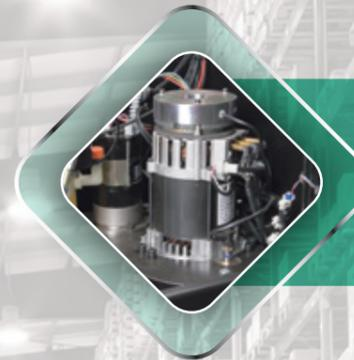
Powerful AC drive motor and state-of-the-art electronics guarantee high productivity with quick acceleration, strong regenerative braking and a high driving speed even with nominal load. Each function can be programmed separately to the application needs and the operator's preference.
