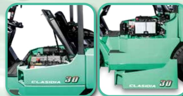
The new Clasidia was designed so that troubleshooting and repairs are easy and require no specialized tools. Access to the engine bay is as simple as pushing a small button and lifting up engine cover. The engine bay is well laid out and there is plenty of room to carry out routine maintenance, service or repairs.
