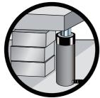
Place blocking or cribbing under the loads as you raise it. Each time you raise it higher, insert more blocking. Position yourself in a manner that will keep you clear of the load, and will not allow your hands or other body parts between the load and the cribbing.
