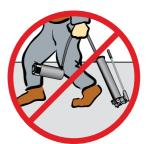
Dragging or carrying rams or pumps by a connected hose can damage the couplers and hoses. Using damaged couplers and hoses can be dangerous.
