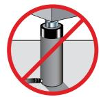
The load must be centered on the ram, or equally distributed on multiple rams. Off center loading can result in the ram slipping out and loss of the load.
