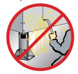
Weld splatter will damage plunger rods and hoses. Hydralic fluid can ignite if vaporized or exposed to high tempertures.
