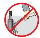
Do not use extensions or cheater bars on hydraulic jacks or hand pumps to raise a load.
