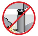
Never attempt to disconnect hydraulic hoses, fittings or couplers under pressure. Unload the ram, open the release screw on the hand pump and shift or open all hydraulic controls several times. If system includes a gauge, double check the gauge to insure pressure has been completely released.
