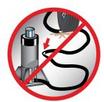
Do not drop sharp or heavy objects on hose. Keep hose out of heavy traffic areas. This will cause internal damage to hose wire strands. Applying pressure to a damaged hose may cause it to rupture. Avoid sharp bends and kinks when routing hydraulic hoses.
