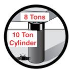
You must know the weight of what you intend to lift and choose a ram with at least 20% more capacity. Be aware of possible load shift requiring more capacity at the particular lifting point.
