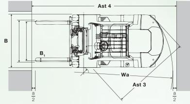
Ast 4 = Wa + X + L<sub>1</sub> + a (a=7.9in/200mm)
