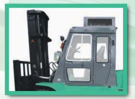
Other optional items include the windshield and wiper as well as airconditioning and heating units. These ergonomic aspects promise an overall comfortable, convenient and safe working space for truck operators.
