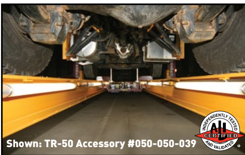
Shatterproof Fluorescent Track Lighting illuminates vehicle undercarriage
