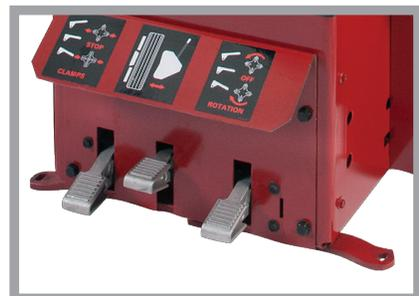
Provides precise control over every step of the changing process. The pedals are ideally placed for fluid technician movements while mounting and demounting tires.
