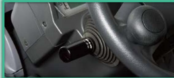
**Electric shift lever** can be moved back and forth at the touch of a finger. (for torque-converter models only).
