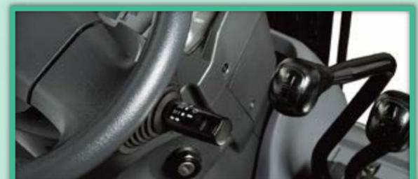
**Combination switch** integrating indicators and headlight switches.
