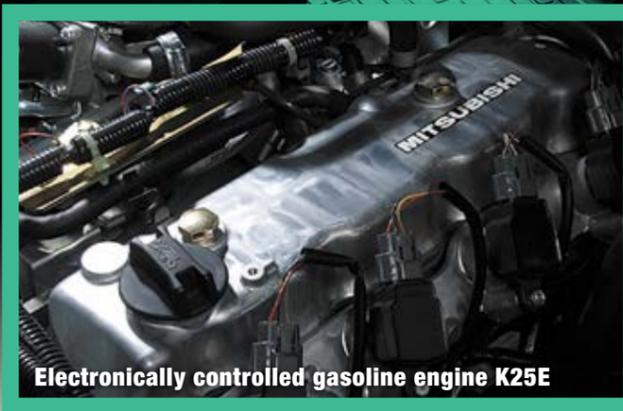
Electronically controlled gasoline engine K25E
