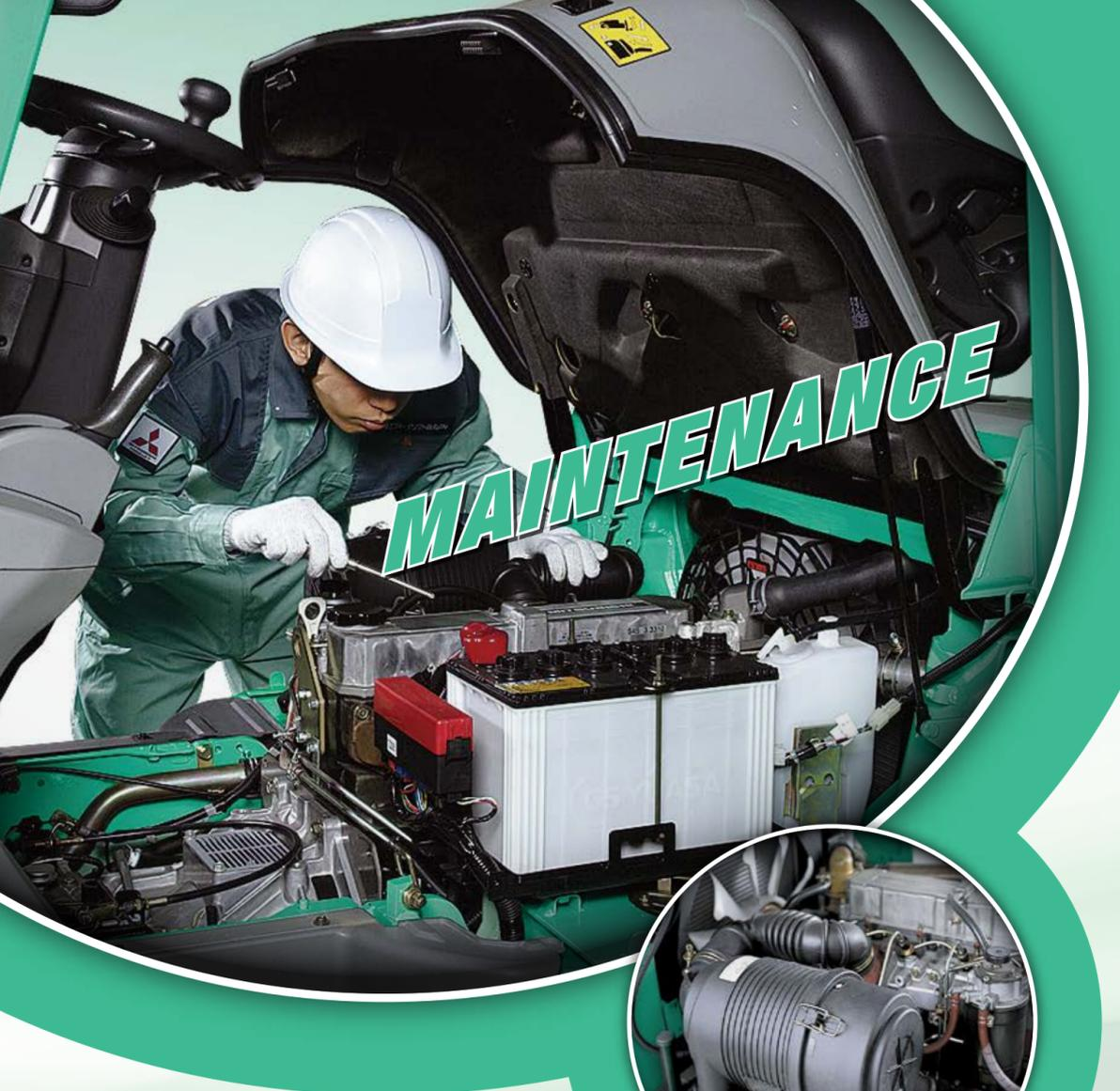
**CENTRALIZED MAINTENANCE POINTS FOR EASY INSPECTION AND MAINTENANCE**
