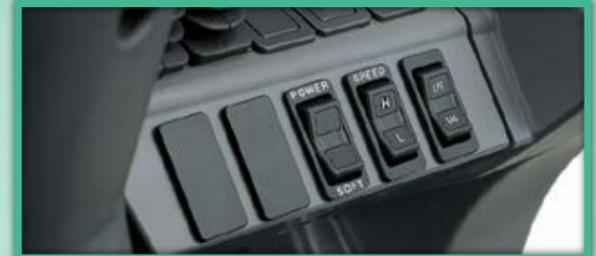
**Switches** for optional functions positioned on the right side of the dashboard.
