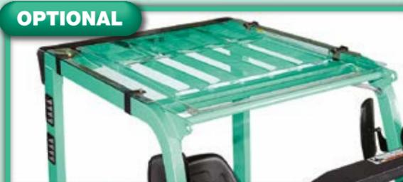
**Acrylic roof** for comfortable operation in outdoor conditions. Easily installed and uninstalled.
