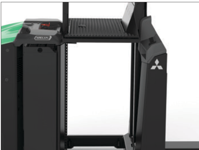
Suspended operator's platform.
