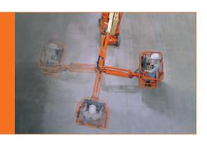
The exclusive JibPLUS° articulating boom option has 180° range of side-to-side movement, providing you with even greater access to hard-to-reach places.
