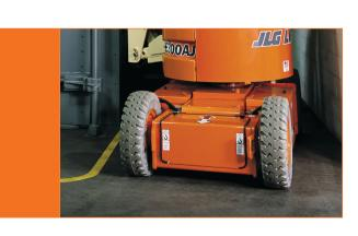
With automatic traction control, both drive wheels work independently for improved traction on uneven surfaces.
