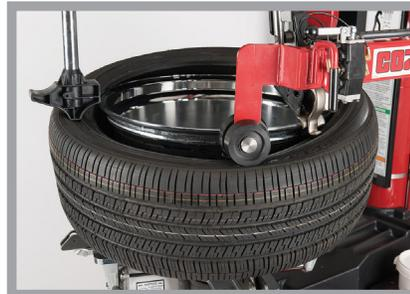
The RoboRoller® provides additional power when mounting difficult tire assemblies by preventing the bead from rolling back over the mount tool.
