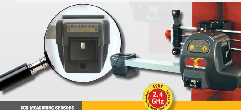
The measuring sensors use the CCD measuring system, and are fitted with 8 sensors for detecting the outer angle edge, the additional measurements, and the real thrust axis of the vehicle. The measuring sensors are electronically levelled.
